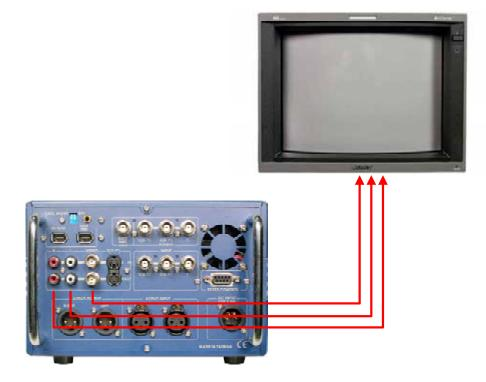
2. Connecting YUV output from the MP-6000 to a Projector.
